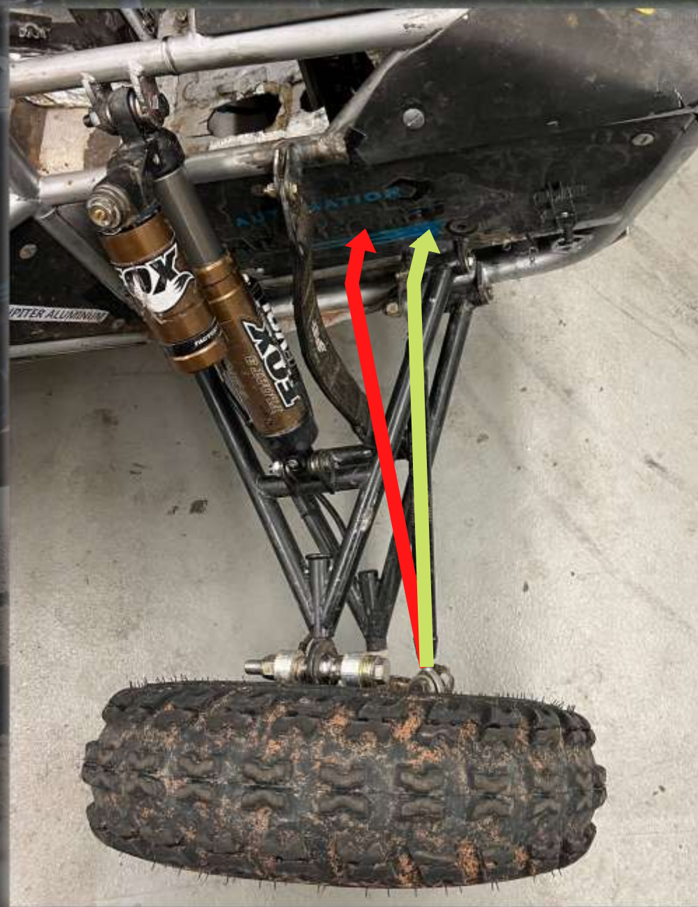
Red: Old Steering Rack Location Green: New Steering Rack Location
